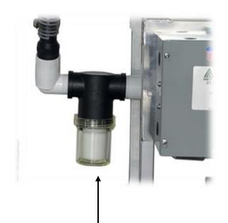
\*ALWAYS make sure that your filter is WHITE & CLEAN, a bi weekly check for discoloration and moisture is highly recommended. These filters are not reusable, do not attempt to clean or alter the filter in any way. Dirty filters should always be replaced every 3-6 months
